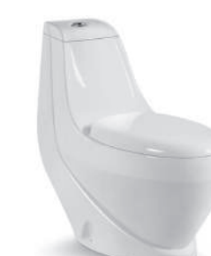
FC-5593 Washdown One-piece Toilet Size: 720x390x750mm S-trap: 300mm Roughing-in
