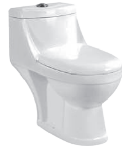
FC-5533 Washdown One-piece Toilet Size: 730x380x645mm S-trap, 100mm Roughing-in
