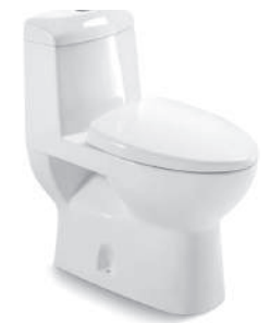
FC-5547 Washdown One-piece Toilet Size: 700x360x680mm S-trap: 100mm Roughing-in
