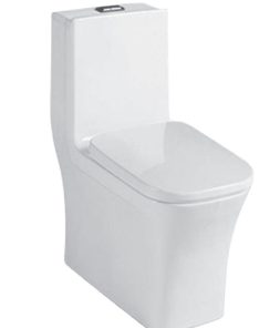
FC-5566 Washdown One-piece Toilet Size: 720x370x800mm S-trap: 180mm Roughing-in
